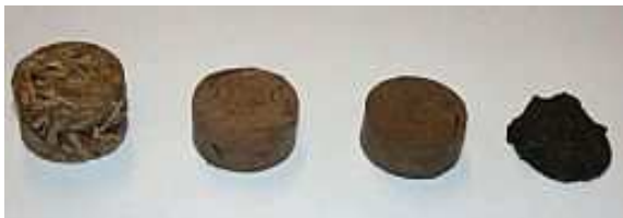
Fuel pellets produced from grass, produced on a laboratory scale TORWASH by ECN
