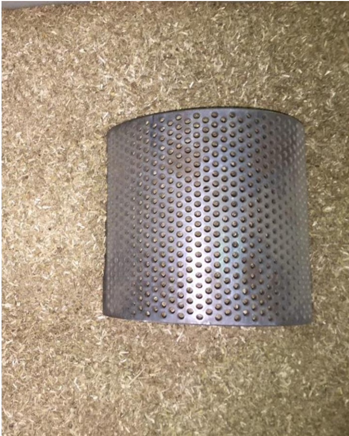
Reed-based particle board; Particles prepared using Wanner cutting mill with 5 mm screen.
